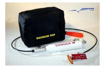
Any position is permissible as an installation position. It should be shot upwards at approx. 10  $^{\circ}$  forwards, if a lateral reject is necessary for constructional reasons, the reject should also be directed at least 10  $^{\circ}$  forwards.
