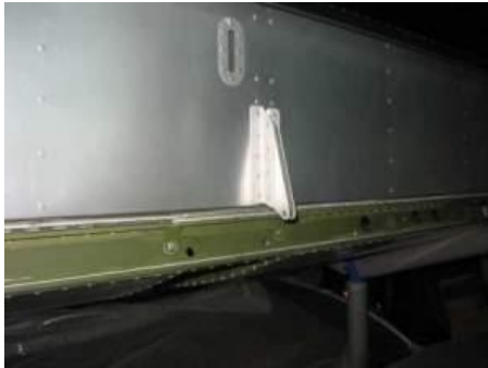
Stabilizer spar Check for distortion and loose rivets
