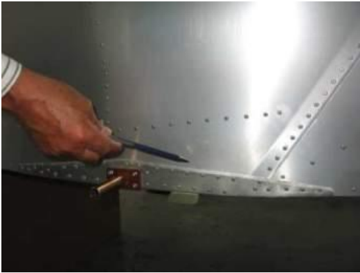
Mid- fuselage reinforcement. Check for loose or missing rivets.
