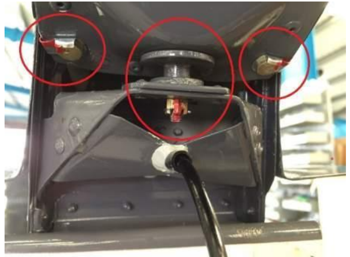
Rudder lower bearing and rudder cable attachment. Check the rudder for end float (max. 0.25 mm) in the attachment bearing and any loose rivets around the attachment point. Check that the rudder cable attachments are secure
