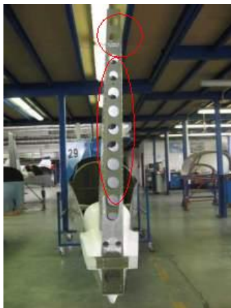
Check the vertical fin spar for distortion and the upper rose joint for security.
