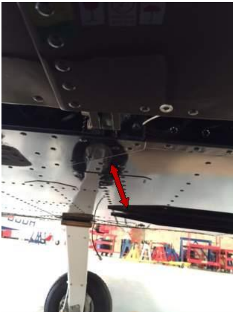
Wing central section rivets. Check for loose or missing rivets where the central spar attaches to the floor.
