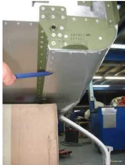
Bottom part of the fuselage under the left bottom engine frame attachment. Check for loose rivets.
