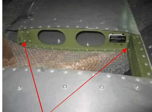
Stabilizer attachment points. Check for distortion, oval or enlarged holes and loose rivets. Attachment point diameters: \varnothing 8+0.04\text{mm} (rear); \varnothing 6+0.03\text{mm} (front).
