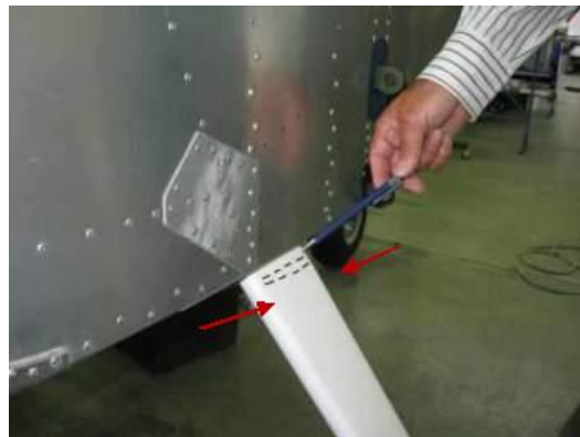
Check main landing gear for cracks across the leg where it enters the fuselage and along the leading and trailing edges of the leg.
