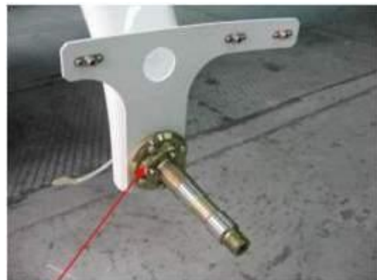
Check the attachment of the wheel axle for security and that the locating pins are not worn.
