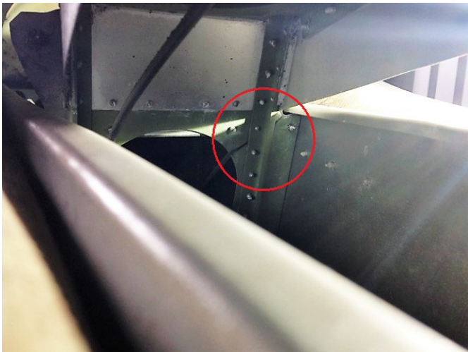
Figure 1 View from rear when the tail plane is removed showing cracked rear fuselage bulkhead.
