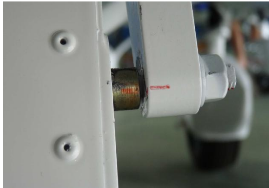
Fig. 3 – Marking the pin position
