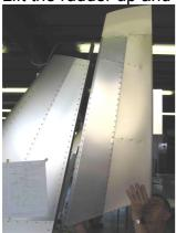
7. Use a slide calliper or another suitable rule to measure distance of the hinge eye rear edge from the fin rear spar and note this value.
