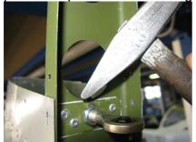
17. Set the rudder back onto the hinges.
