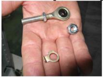
10. Set a new tab washer (size 8) onto the hinge thread. It is not recommended to straighten up and use original washer, due to possible cracking when being bent repeatedly.
