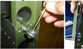
9. Pull out the hinge, self locking nut and tab washer.
