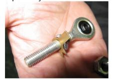
11. Set the hinge back on the fin spar, the washer must be on the outside of the spar as shown on the picture.
