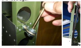
9. Pull out the hinge, self locking nut and tab washer.
