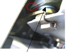
Note: The two "normal" washers above the cable ends are installed to prevent cables from being chafed from the rudder front lower edge (marked red). Installation of these washers is recommended if not installed and there is an evidence of chafing in this area.
