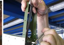
13. Measure the distance between hinge eye rear edge and fin spar and if different from the original one, then screw or release the hinge to adjust this distance.
