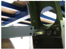
8. Screw M6 nut on a sufficiently long M6 bolt (80 mm), then put a washer (25 mm diam.) on the bolt and insert into the hinge from above. Put another washer on the bolt from below and tighten with another M6 nut. Now set M13 nut wrench through a lightening hole on the self locking nut inside the fin (right figure below) and turn the M6 bolt to release and unscrew the hinge.
