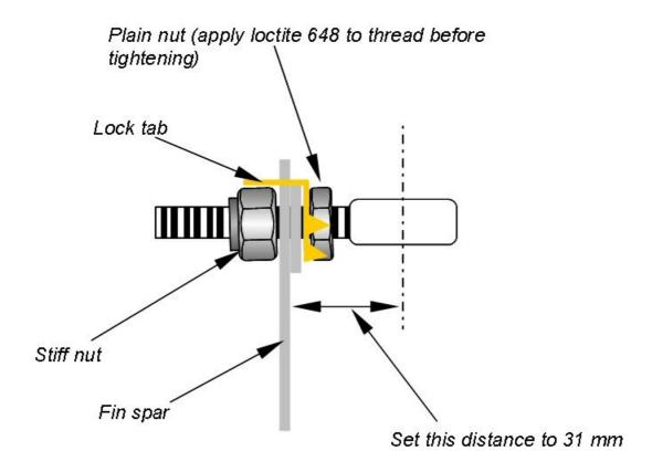
As the rudder is a primary control, a dual inspection of the finished job will be necessary. Record the work in the aircraft log book and keep a copy of this bulletin in the aircraft records.
