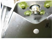
19. Set new tab washers (size 6) on the cable attachment screws.
