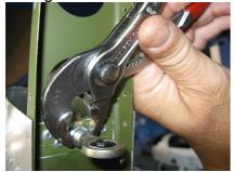
16. The washer bigger tab must be bent forward by a suitable tool (e.g. flat screwdriver and hammer) to protect the washer from rotation. The end of bigger tab should be pressed up to the self-locking nut edges.
