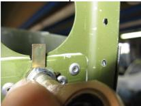
12. Screw the self locking nut (it has steel core so can be re-used) and turn it several times to be fixed on hinge thread. Then follow step 8 to install M6 bolt, washers, and nuts. Turn the bolt clockwise to screw down the hinge eye.
